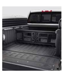
Includes cargo rail system with four adjustable tie-down loops, a deployable bed step and spray-in bedliner, that provides seamless, durable protection with a special finish that maximizes bed resistance. The models with Rambox are equipped with a bed divider.
