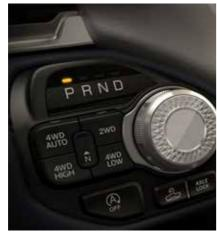
Starting from the Big Horn trim, it includes the Auto mode, which instantly transfers torque to the front only when needed, ensuring minimal fuel consumption and maximum safety.
